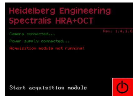
Once a patient file is open and entries for an acquisition are made, the Acquisition Window with the live image will open (see chapter 3.6 “Acquisition Window” of the Software Operation Manual), and the ‘Start/Stop’ button (0), on the “System Start” screen of the Control Panel will change from red to white. Press the white ‘Start/Stop’ button in order to turn on the laser.
