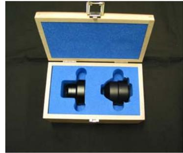
The optional 55° wide angle lens for IR, RF and angiography wide-field imaging is mounted the same way: it has to be inserted with the red dot orientated upwards (12 o'clock) and then rotated by about 50° clockwise until it snaps in.
