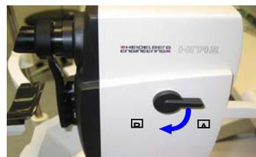
NOTE: When the filter lever is not properly locked in to one of the above positions, it will not be possible to acquire any images. A notice to this effect will appear at the bottom of the acquisition screen.
