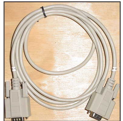
RS485 Communication Cable(s)
