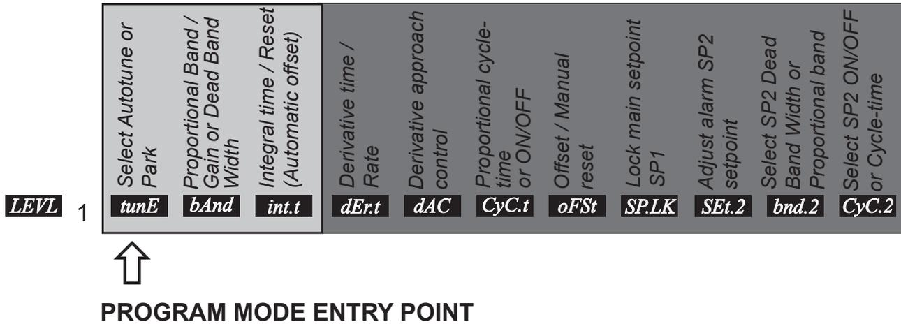
All controls and functions are located in program mode. To enter program mode on the controller, push the **up** and **down** buttons at the same time for 3 seconds until the **tunE** function appears. Once **tunE** is displayed, the controller is in program mode. Within the program mode there are multiple levels, and within each level, there are multiple functions within that level.
