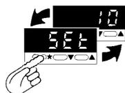
In work mode, press and hold the \* button. Setpoint is shown in alternating display.
