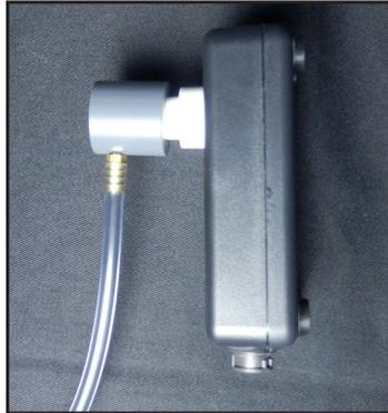
3. With the calibration chamber connected, open the **GAS BLEED** valve knob on the front panel of the ProOx model 360 unit until gas is heard expelling slightly through the calibration chamber.
