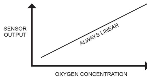
Sensors generate an electrical signal (output) which is linear and directly proportional with the gas concentration.
