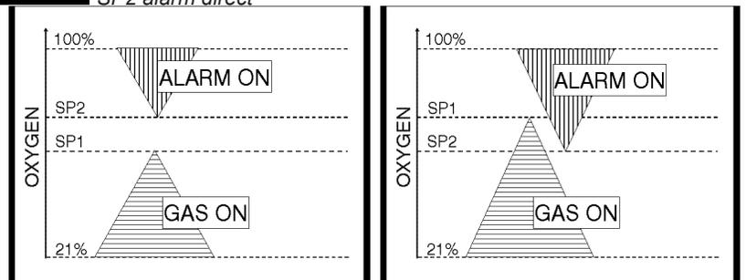
The controller has two output modes which are located in the *rEV.d* function in Level 3. Direct output (1d) is used for low oxygen control, generally under ambient air (21%). Reverse output (1r) is used for high oxygen control, generally above ambient air (21%). The output mode programmed is predetermined at the factory based on customer specifications.
