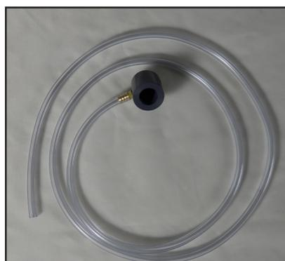
**Calibration Chamber with Tubing**
