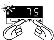
Simultaneously hold both **up** and **down** buttons for 3 seconds. Program mode is entered from normal operating mode at **tunE** function on **LEVL 1**. Exit program mode at any point in the menu, returning to normal operating mode. With exit, any new instructions get entered into the memory.
