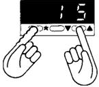
Index to required function. Press and hold the \* button (current option displayed). Press **up** and/or **down** buttons to display new setting. Release the \* button. **IMPORTANT:** Check new selection (alternating with function) before moving to another function or exiting program mode.
