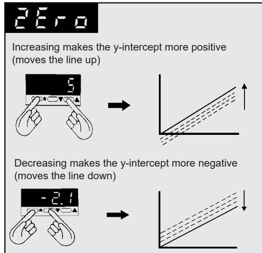
The **SPAn** function adjusts the slope of the line, but does not affect the Y-intercept (set by **ZERo** function). Always do **SPAn** after **ZERo**.
