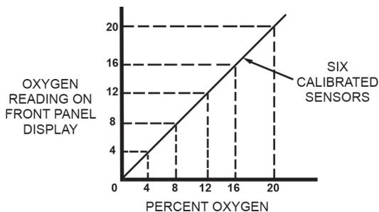
Check calibration as frequently as necessary to have confidence in accuracy. Weekly checks are usually sufficient. Check before and after each experiment.
