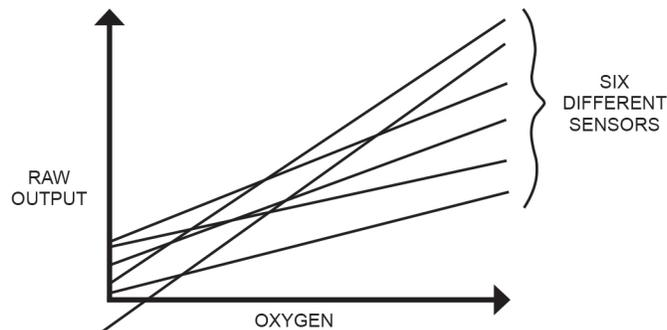
Sensor output changes over time (drift), generally but not always in a slow, downward direction. Sensors remain linear but gradually lose power. Some sensors drift more than others.
