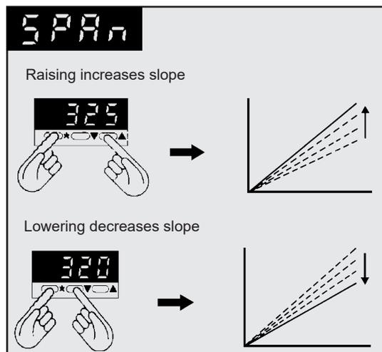
**REMEMBER:** Never adjust the **ZERo** function without adjusting the **SPAn** function afterwards. **ZERo** affects **SPAn** setting, but **SPAn** does not affect **ZERo** setting.
