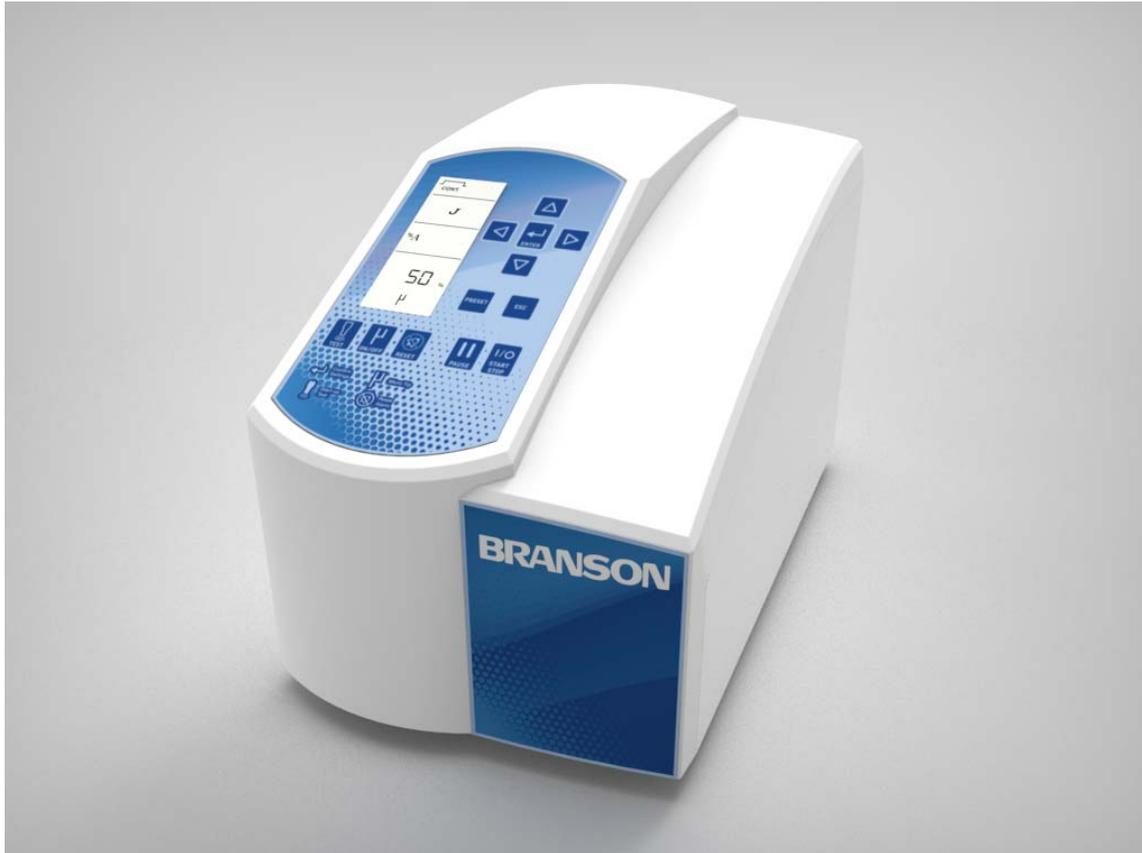
The Sonifier power supply converts AC line voltage to 20 kHz or 40 kHz electrical energy. This high-frequency electrical energy is fed to the converter where it is converted to mechanical vibrations. The heart of the converter is an electrostrictive element which, when subjected to an alternating voltage, expands and contracts. The converter vibrates in a longitudinal direction and transmits the motion to the horn tip immersed in the solution, which causes cavitation.
