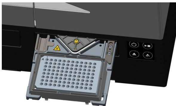
Figure 97: Microplate on the plate carrier with the A1 well in the upper left-hand corner
