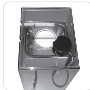
4. Place the waterbath into the sound-proof box and add the accessory.
