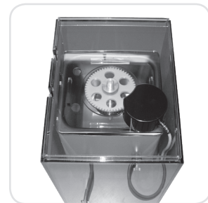
4. Place the waterbath into the sound-proof box and add the accessory.
