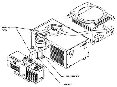
Be sure to use the proper cartridge for your application. When the media in the insert has changed color, discard the insert and replace it with a new insert. For the radiochemical trap insert, no color indicator exists therefore it should be discarded after each use. Use a Geiger counter to monitor the pump exhaust.
