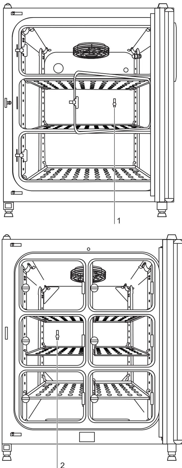
Fig. 73: Gas-tight screen measurement opening
