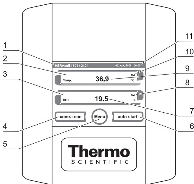
Fig. 32: iCan™ touchscreen without O<sub>2</sub>/N<sub>2</sub> gas supply
