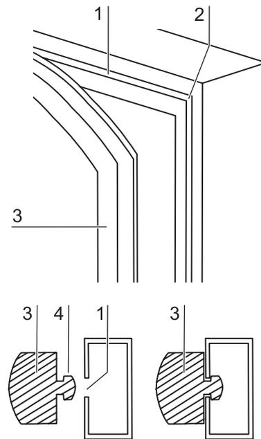
Fig. 77: Magnetic door seal replacement
