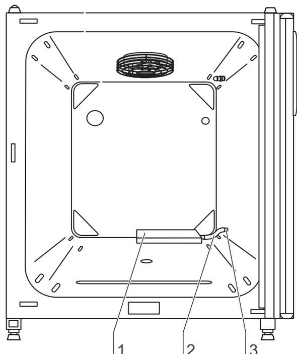
Fig. 20: Installing gas humidification
