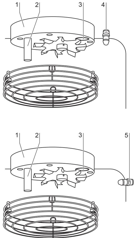
Fig. 11: Temperature, CO<sub>2</sub> and O<sub>2</sub> sensors
