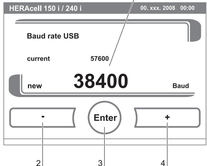
Fig. 46: USB interface baud rate setting
