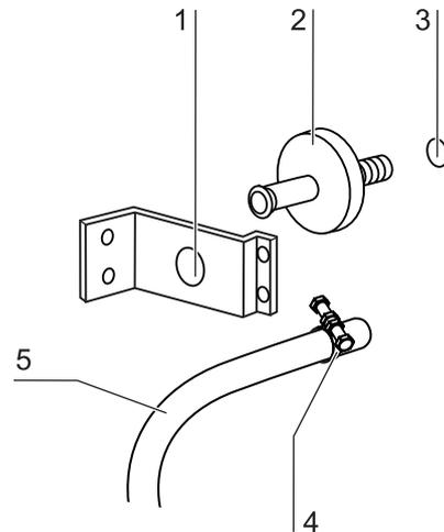
Fig. 75: Gas inlet filter installation
