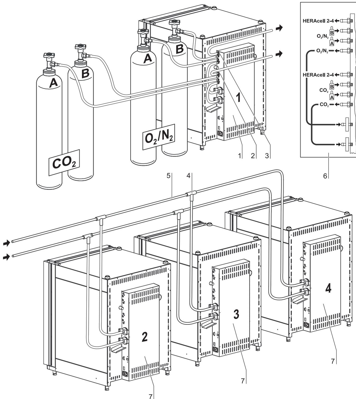
Fig. 6: Looped-through gas supply
