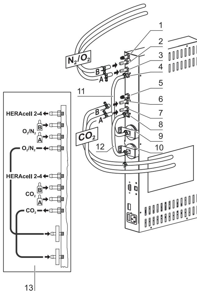
Fig. 27: Combined connection with gas monitoring system (optional)
