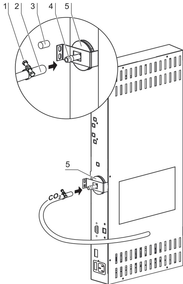
Fig. 24: Installing gas pressure hoses
