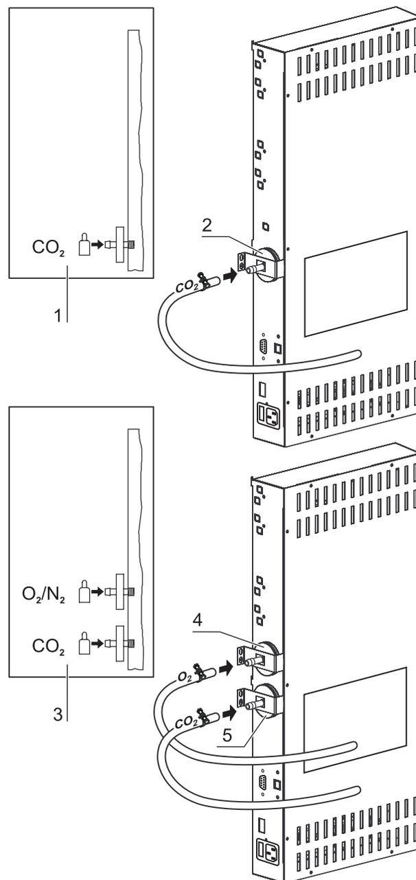
Fig. 25: Gas connection without gas monitoring system
