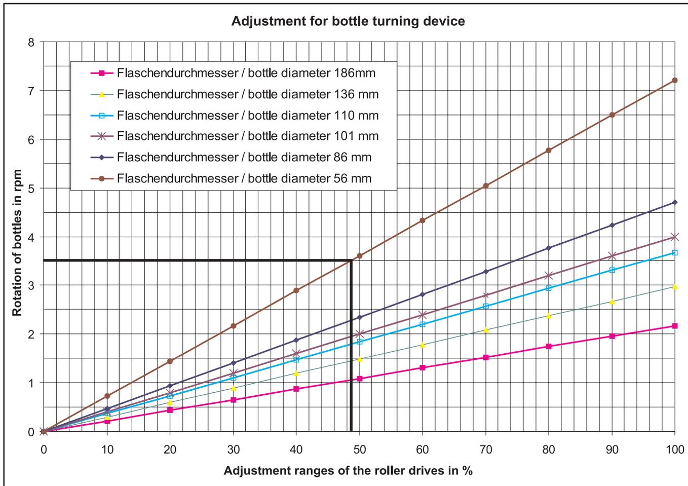
Fig. 22: Bottle turning speed
