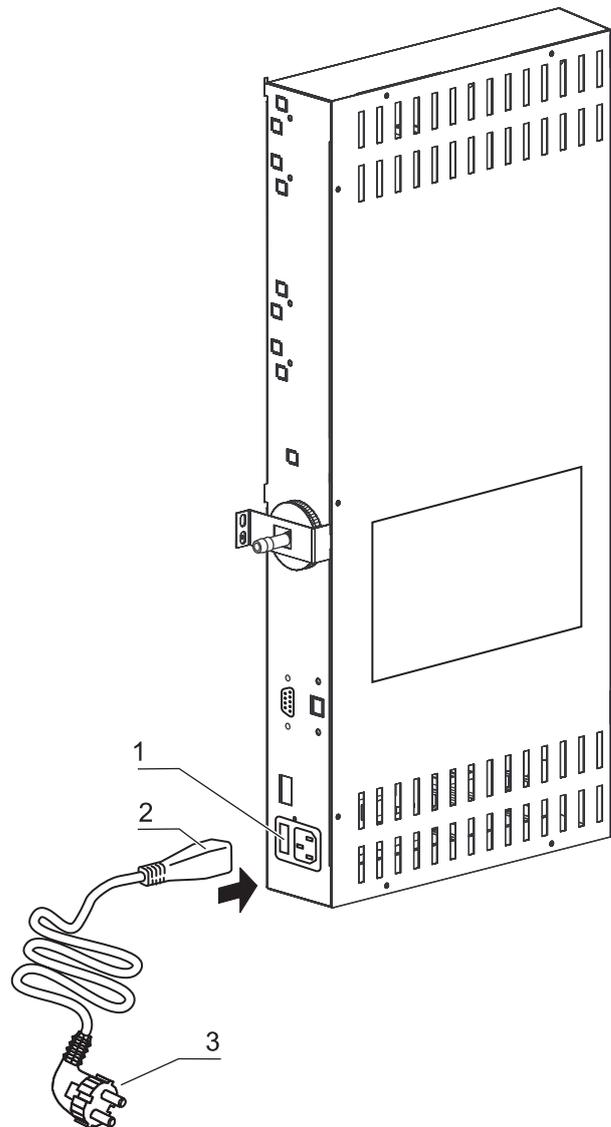
Fig. 28: Power supply connection
