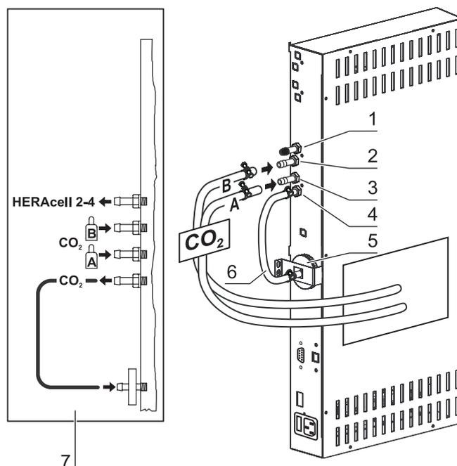
Fig. 26: Gas connection with gas monitoring system (optional)
