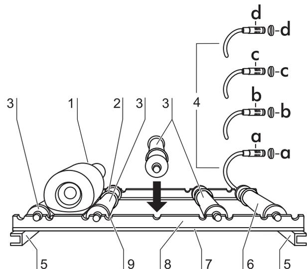
Fig. 21: Installing the bottle turning devices
