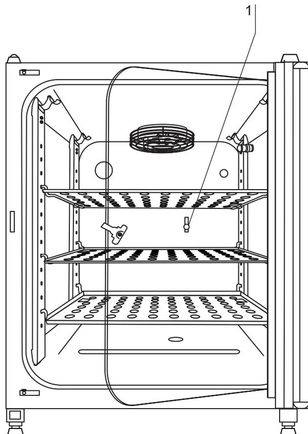
Fig. 72: Preparing CO<sub>2</sub> calibration
