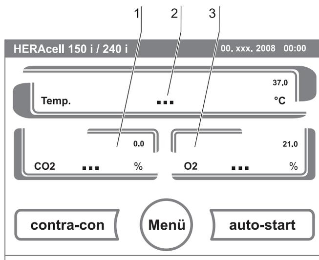
Fig. 35: Heat-up phase display
