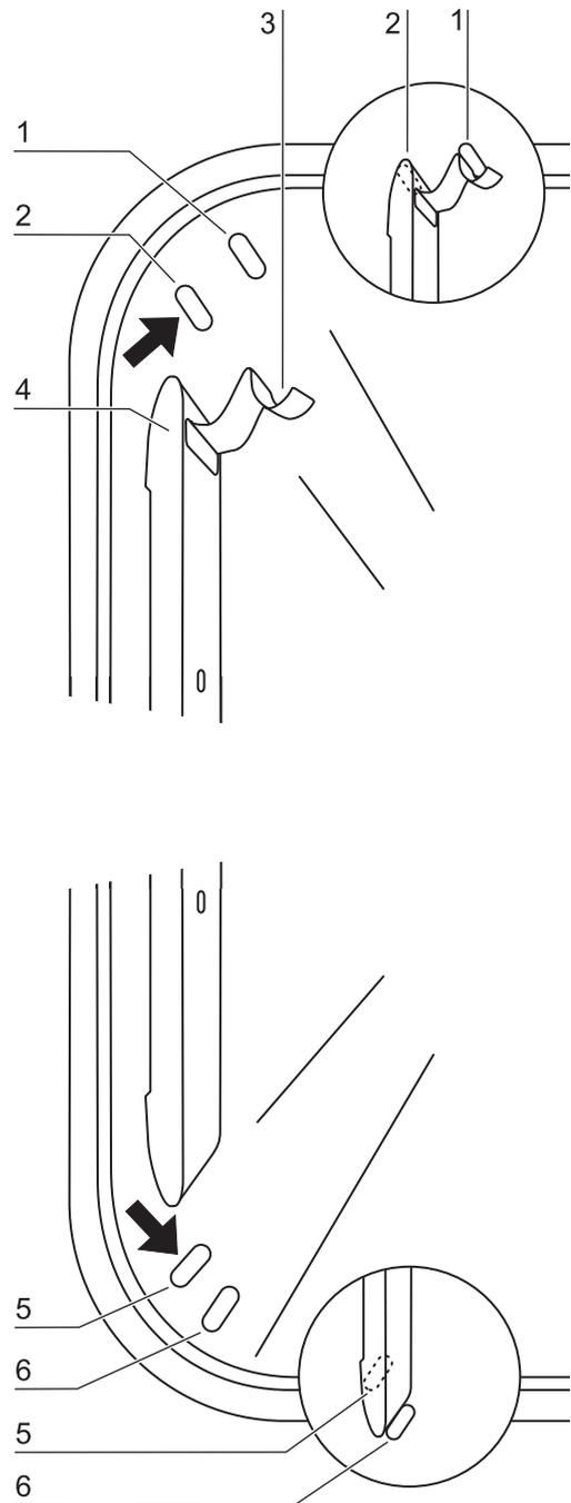
Fig. 18: Support rail installation/removal
