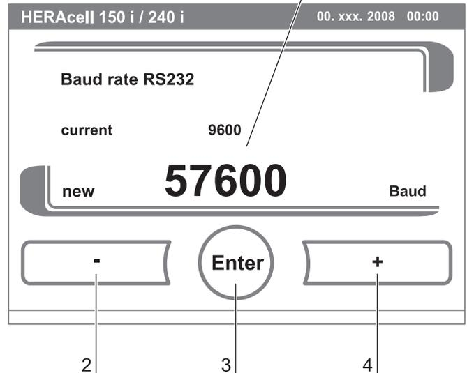
Fig. 45: RS 232 interface baud rate setting
