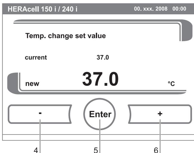
Fig. 36: Setting the temperature set value
