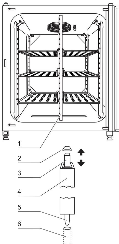
Fig. 23: Center strut installation
