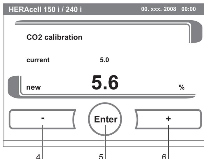
Fig. 74: CO<sub>2</sub> calibration procedure
