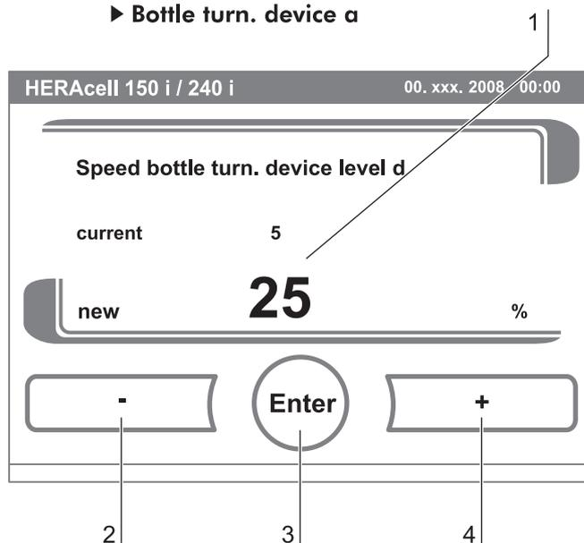
Fig. 57: Bottle turning device speed setting
