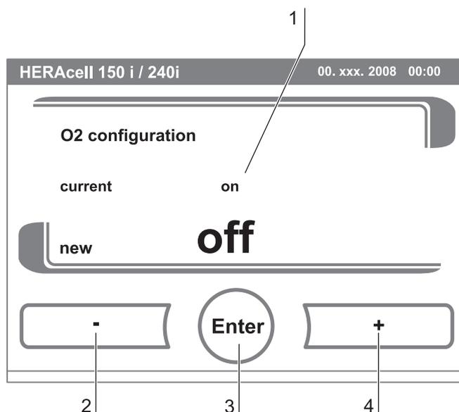
Fig. 58: Switching the O<sub>2</sub> control on and off
