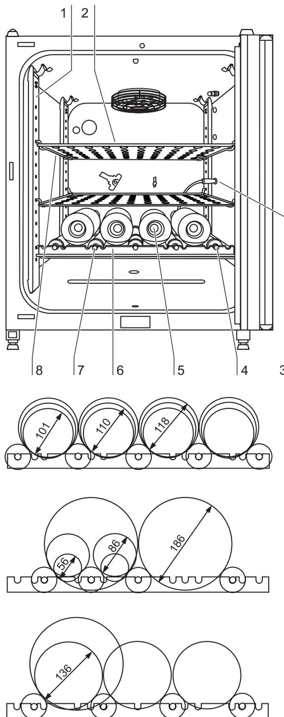
Fig. 16: Bottle turning device
