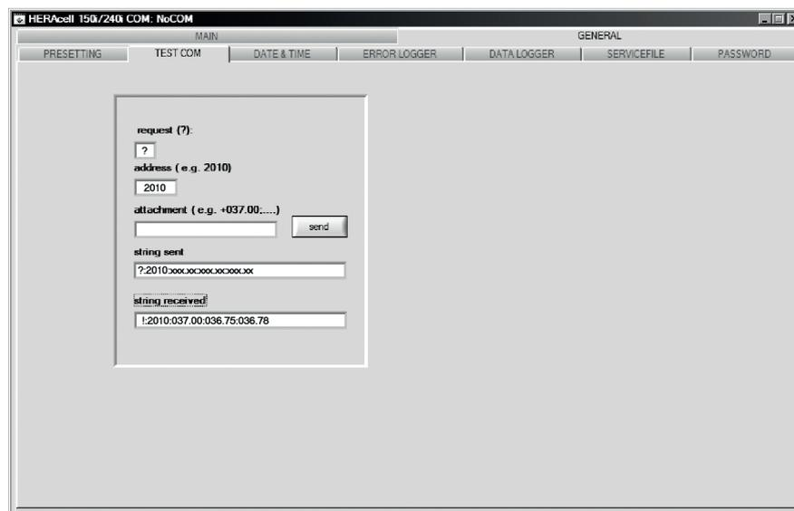
1. Example of a query for the currently measurable temperature values of the incubator:
