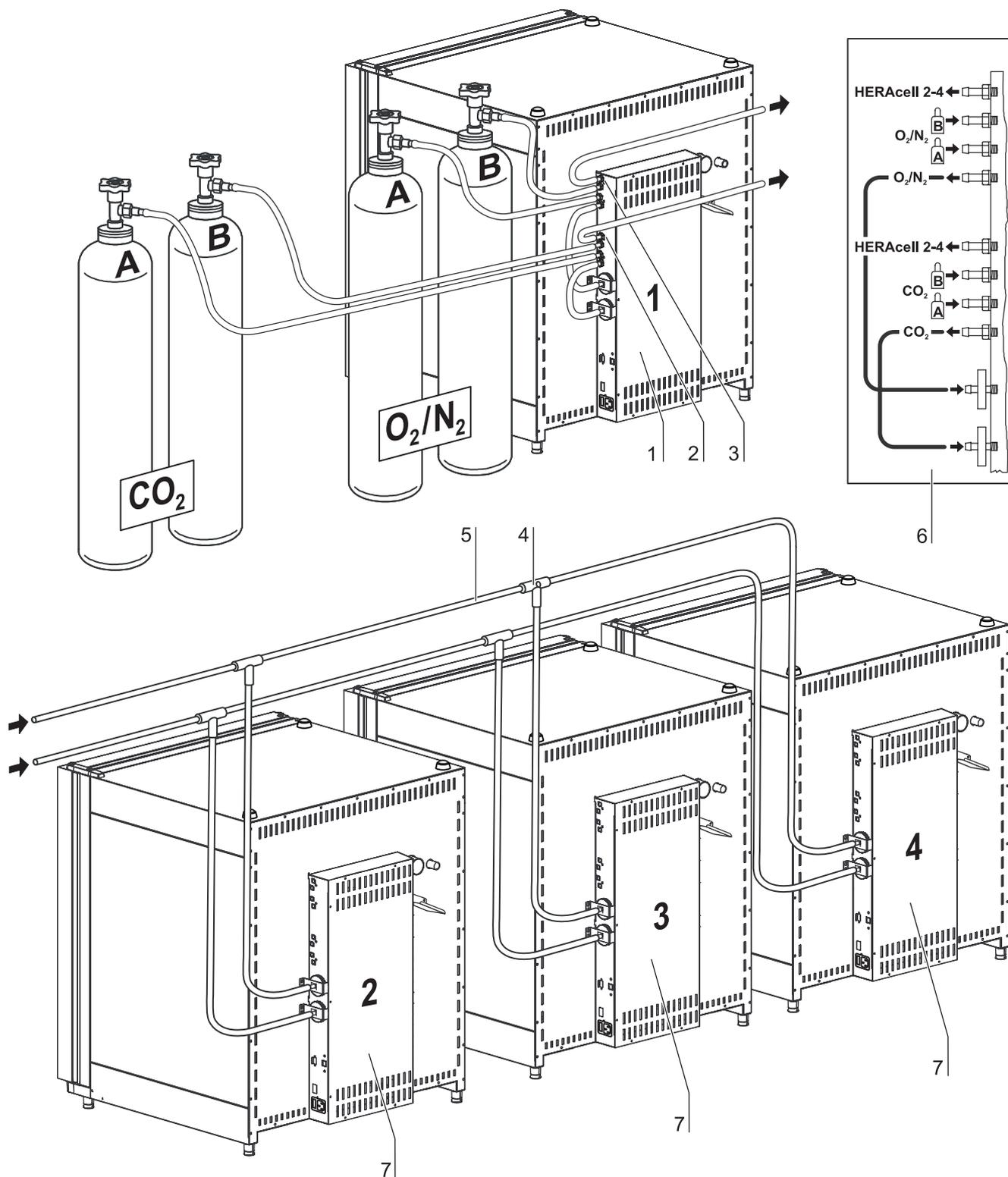
Fig. 9: Looped-through gas supply
