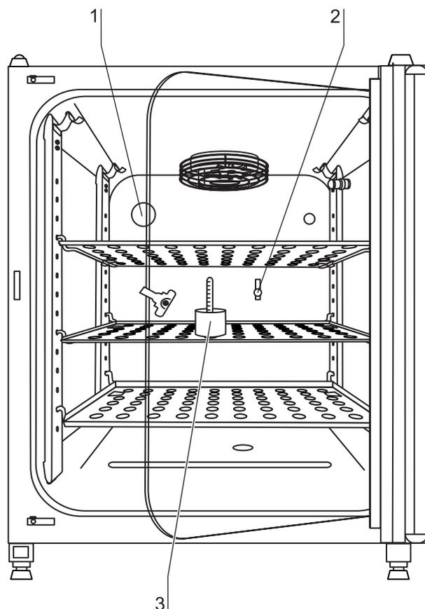
Fig. 70: Preparing the temperature calibration
