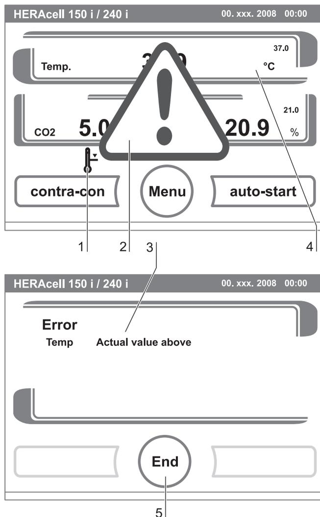
Fig. 65: Event error overtemperature
