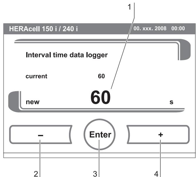
Fig. 50: Logging cycle setting
