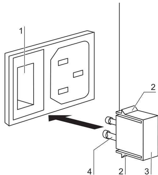
Fig. 76: Device fuse replacement
