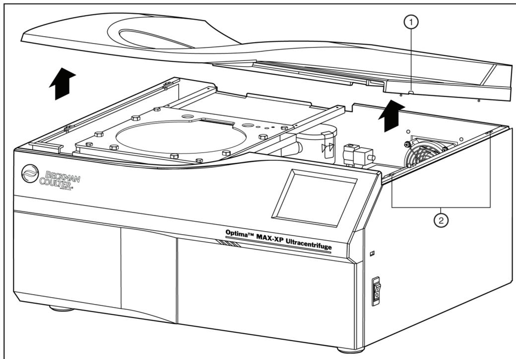
1. Release slot (located on right and left sides)    2. Clips for securing cover
