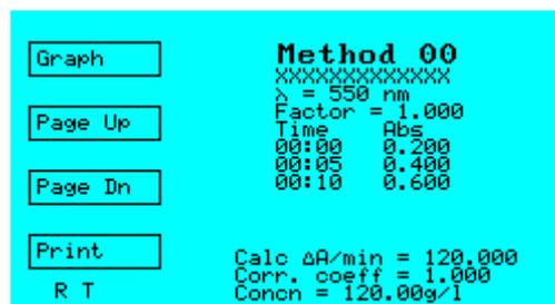
The  $\Delta A/\text{min}$  is calculated using a Least Squares Fit. You can view the graph by pressing Function Key 1, or scroll through the readings using the page up or page down keys.
