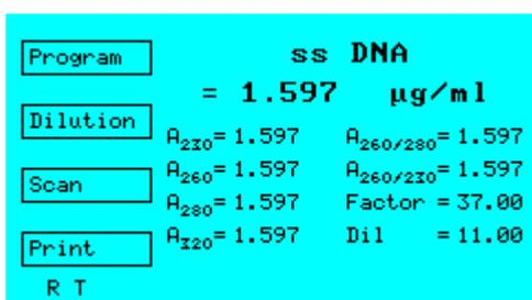
The ratio readings give information about the purity of the sample. The A260/230 reading give a measure of phenol contamination following extraction .
