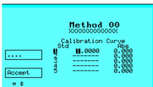
Press Accept to confirm. Once all the standard values are correct, press Function Key 4 "All OK".
