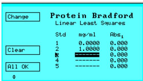
Press change to modify the standard value. The cursor keys allow the digits to be changed - move to the next digit using  $\leftarrow\rightarrow$ . Function Key 3 "....." moves the decimal point by one space when pressed.
