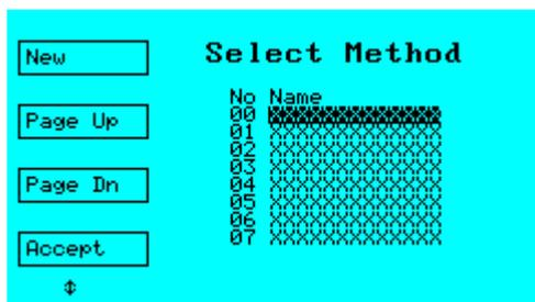
To select a method, move the cursor to the desired number using the Page up or Page down functions and the arrow keys and then click on "Accept". Alternatively select a new method to bring up the next free location.
