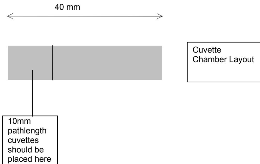
**Note:** It is important to align the square cuvettes to the left-hand side of the chamber. The alignment of the cuvette is important to ensure reproducible readings.
