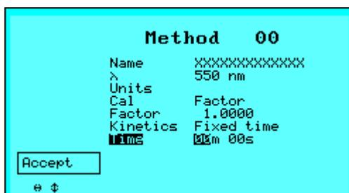
This allows the user to set a timed delay before a measurement is made. This is suited to tests where the final result depends upon allowing the sample to react for a certain length of time and is especially useful where the Absorbance is likely to attain a certain value and then decay.
