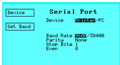
The Biowave has a bi-directional RS232 port that can be used to connect to a PC or 40-column printer.
