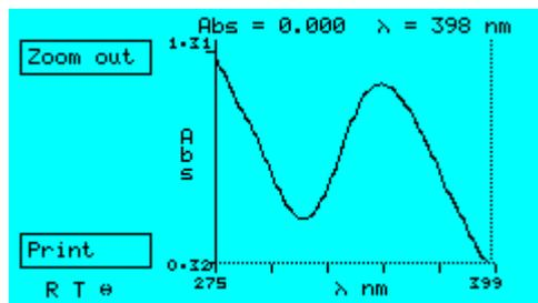
The spectrum is automatically re-sized to fill the screen. The cursors can be used once again to identify the reading at a particular wavelength.
