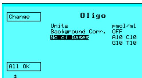
Pressing Change allows the No.of Bases to be entered using the cursor keys in the normal manner (similar to Dilution Factor).
