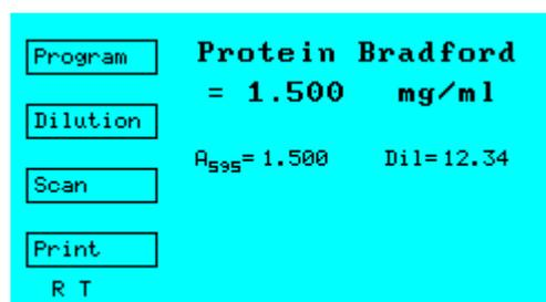
The program button allows the units of concentration to be changed , and the calibration between standard and factor to be selected .
