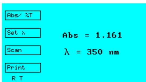
This mode should be used when readout in Absorbance or %Transmission is required for a single wavelength.
