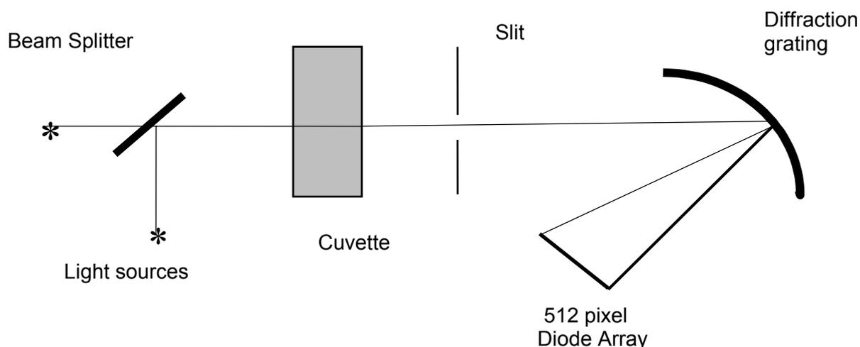
***The added advantage of the above optical arrangement is that Stray light is minimised, thereby eliminating the need for a cover over the cuvette chamber.***
