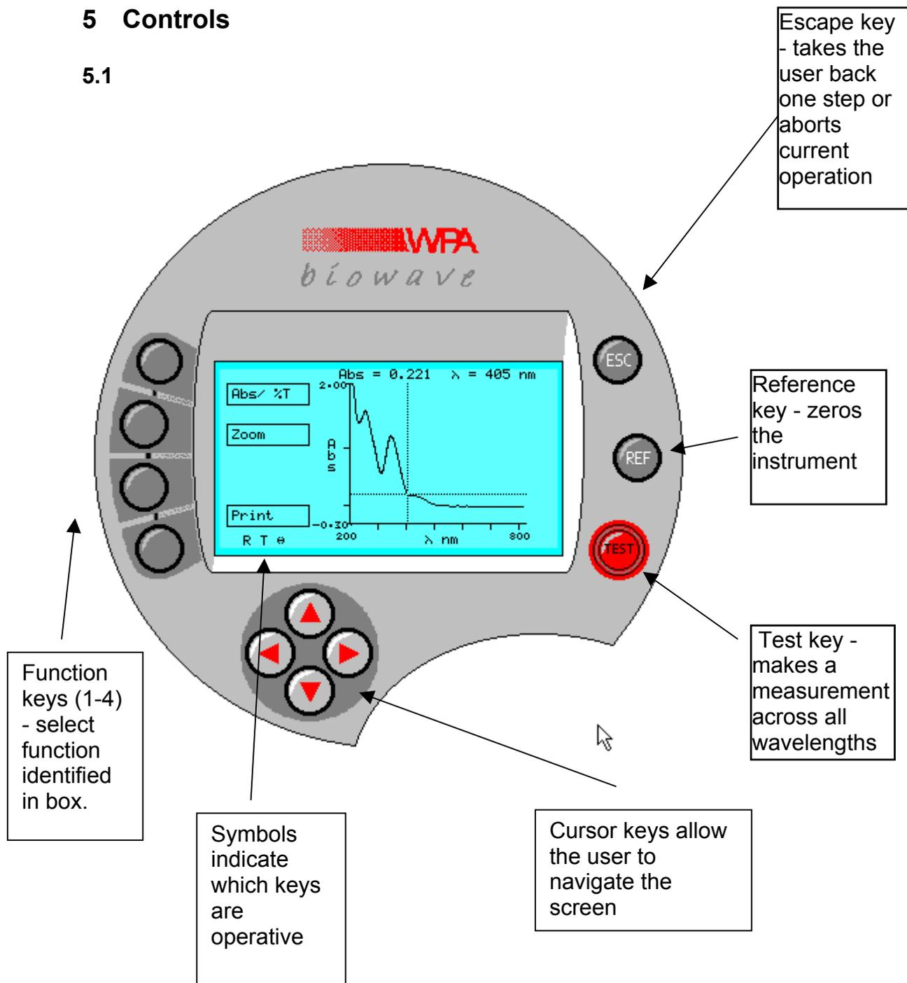
Note: The arrow keys and REF and TEST buttons are only operational in certain modes. When operational, symbols (R for Ref, T for Test, + arrows) will appear in the bottom left hand corner of the display. Similarly the Function keys on the left-hand side of the display are only operational when a box appears.
