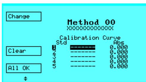
Press change to modify the standard value. The cursor keys allow the digits to be changed - move to the next digit using ←→. Function Key 3 "....." moves the decimal point by one space when pressed.
