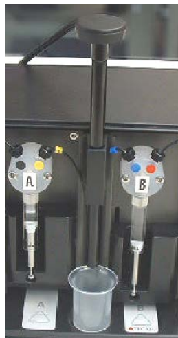
Figure 43: Injector-box with injector in 'service position'; the injectors are removed from the carrier slot and inserted into the holder of the injector carrier system.
