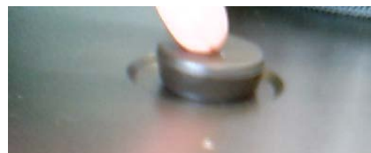
Figure 7: Inserting the injector carrier into the injector port
