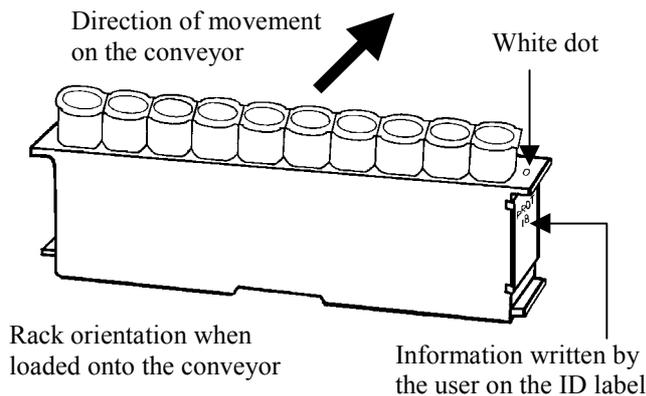
Rack orientation when loaded onto the conveyor
