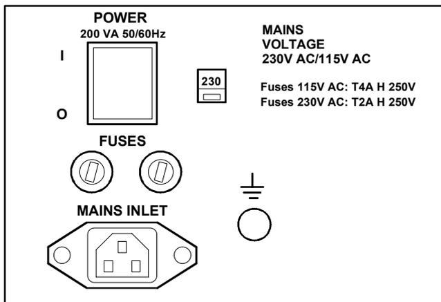
The mains selector in older instruments has the voltage marked on it and is combined with the fuse carriers. To adjust the mains selector, pull it out, turn it through 180 degrees and replace it.
