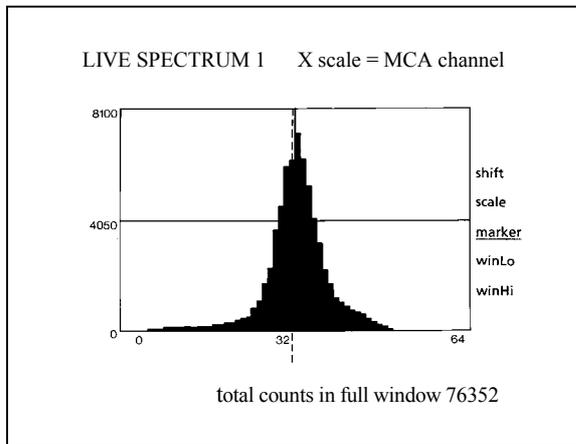
On the right hand side of the spectrum five functions are displayed. By using the up and down arrow keys you can select the function you want. A function is shown to be selected by the underline mark appearing under the function name. The functions are as follows:
