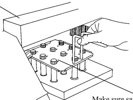
Make sure samples are loaded according to numbers on tray
