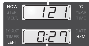
Sterilization remaining time or melting remaining time (after the temperature reaches the sterilization temperature or melting temperature)
