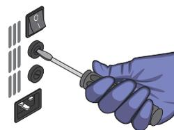
3. Remove each fuse from its fuse holder and inspect it for damage. Carbon typically coats the inside of failed fuses.
