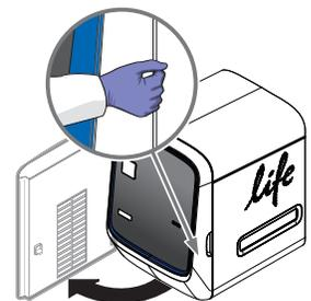
3. Firmly press down on the handle of the sample block, then remove it from the QuantStudio™ 12K Flex Instrument. Place the sample block on a clean, dry surface.
