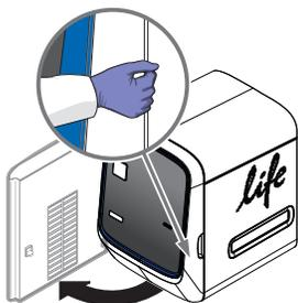
4. Firmly press down on the handle of the sample block, then remove it from the QuantStudio™ 12K Flex Instrument. Place the sample block on a clean, dry surface.
