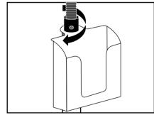
2.Place gooseneck over metal connection then turn clockwise to screw down until tight.
