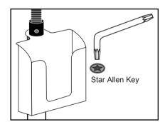
3.Use the smaller Star Allen key to tighten the small star meter screw inside the gooseneck. Note: if meter screw is already in, unscrew before attaching gooseneck in step 2.
