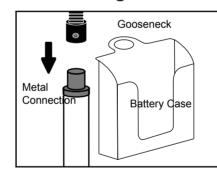
1. Place battery case over metal connection on the pole
