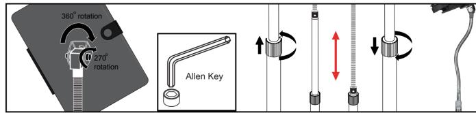
1.Use included Allen key to tighten and loosen the gooseneck to holder connection screw to adjust ease of rotation.
